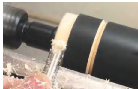
▲ Pic.21 The other benefit of the 10mm skew is that you can cut spigots and tenons much quicker than you can with a parting tool
